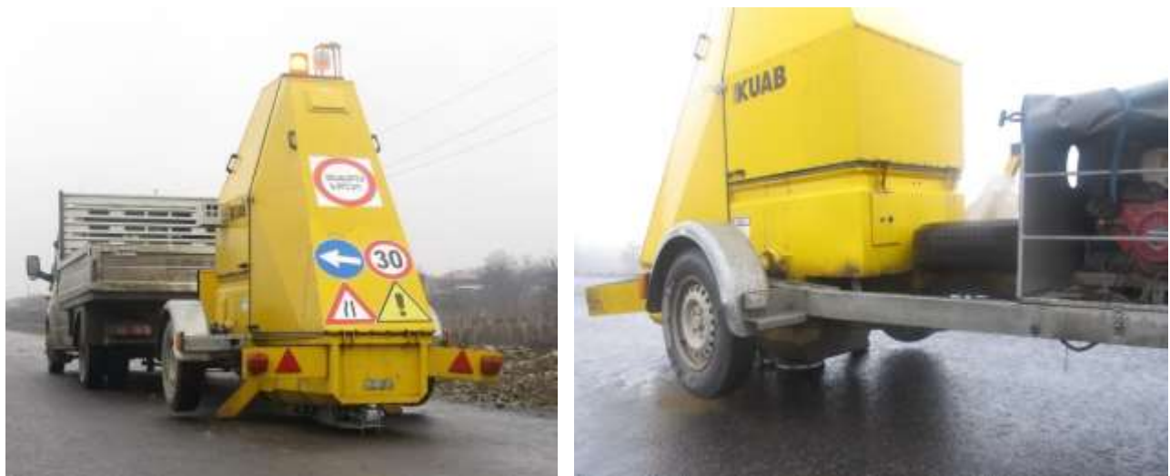
Pic.1. Falling Weight Deflectometer FWD KUAB 50 during testing
