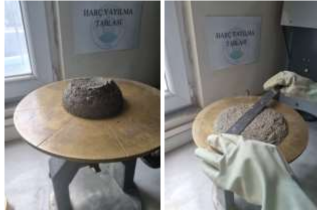
Figure 2. Flow table test
