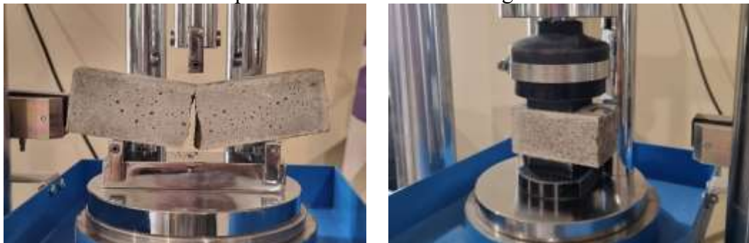
Figure 3. Flexural and compressive strength test
